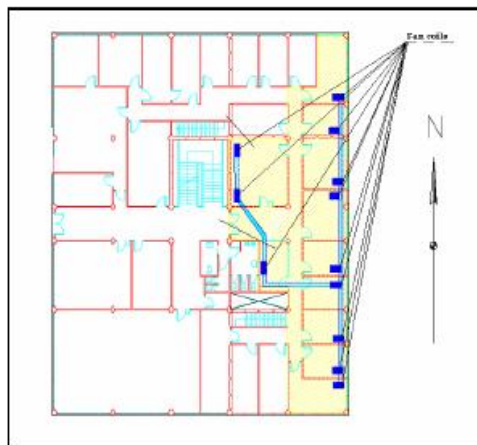
Figure 6- Fan coils distribution scheme.
