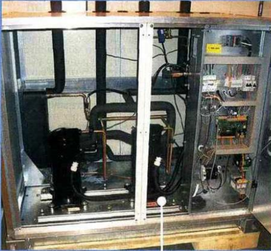
One heat pump, two compressors The calculations have shown that it is better to use two small compressors running in stages than one bigger running in variable speed.
